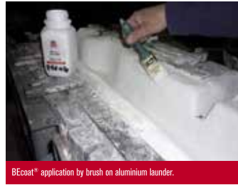
Launder treated with BEcoat®, ready to be put into operation.
