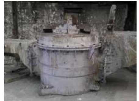
Photo 4 - Second ladle lined with Eredi Scabini solution.
