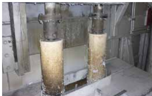
Flextrong® HT AL impellers after 15 days in operation.
