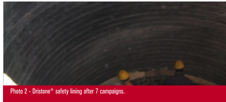
Photo 2 - Dristone® safety lining after 7 campaigns.
