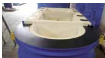
Working lining in Ultrablock® and 2lite® for insulation.
