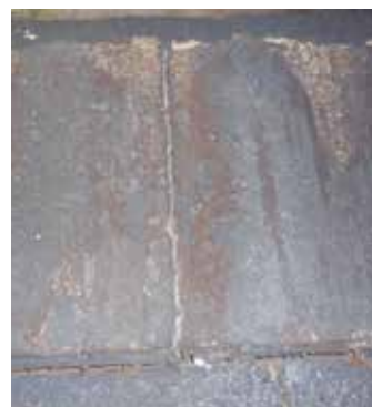
Photo 12 - Eredi Scabini Solution, joints in blocks after 12 months.
